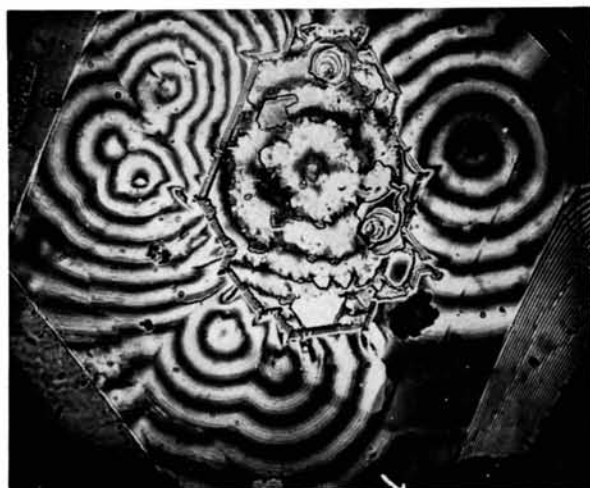
Fig. 5. Micrograph of (0001) with interference fringes on crystal No. 26. Mag. \times 320 .
