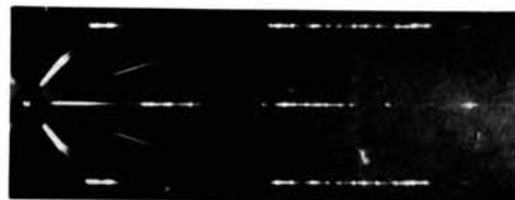
Fig. 13. 15°-oscillation photo about a axis of crystal No. 59 (Cu K\alpha , 3 cm. camera). Mag. \times 1 .
