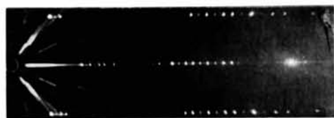
Fig. 4. 15^\circ -oscillation photograph about a axis of crystal No. 46 ( Cu K\alpha , 3 cm. camera). Mag. \times 1 .
